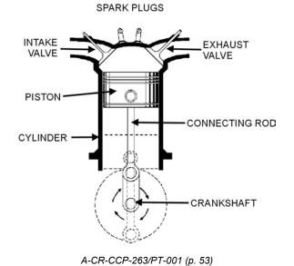
Figure A-4 Piston-powered Engine Schematic
