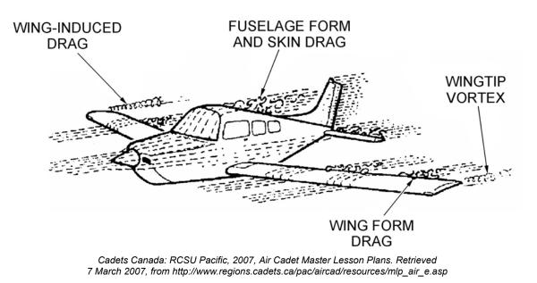
Figure D-1 Types of Drag on an Aircraft
