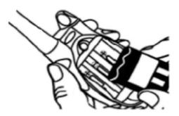
Motorola Inc., Talkabout FRS/GMRS Recreational Two-way Radios Models T5000, T5500, T5550 User's Guide, Motorola, Inc. (p. 13) Figure 4 Changing the Batteries
