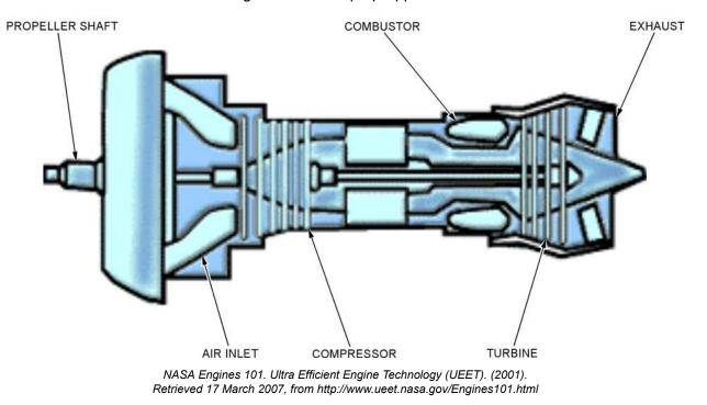
Figure A-10 Turboprop Engine Schematic
