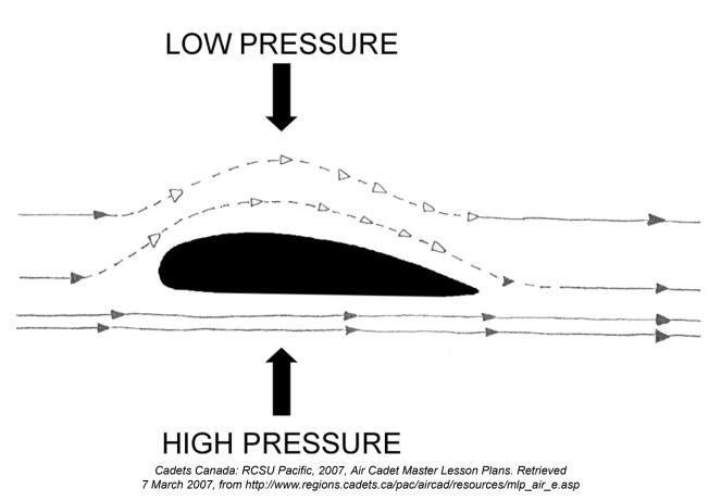
Figure C-1 Lift from an Airfoil
